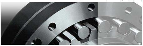
In this type of freewheel, the two races are cylindrical. The sprags, fitted in a cage, feature an active profile that ensures engagement or disengagement according to the relative motion of the races. It is possible to adapt the design of sprags and cage to get significantly different characteristics from one model to another. For example, models which have permanent contact or are contact free during overrunning, are available.
